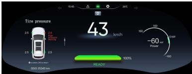
When the vehicle is driving at a speed of  $\geq 25\text{km/h}$  and continues for a period of time, the instrument cluster assy can display tire air pressure in real time.
