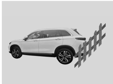
2. The radar probe cannot detect low objects such as rocks.
