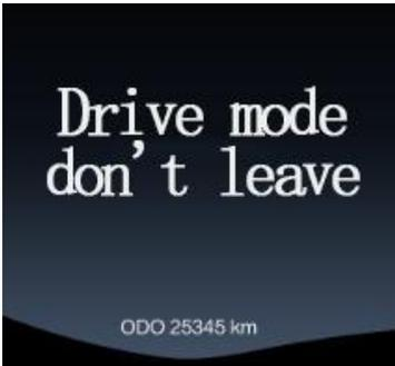
When the vehicle is in D gear or S gear or R gear and the left front door is opened, it will prompt "Driving mode, please do not leave" for 5S, accompanied by three beeps. Prompt Message13: Position light is not turned off warning
