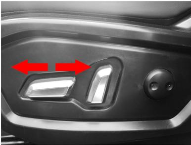
Adjust seat button1 in the direction shown in the figure to adjust the front and rear of the seat as a whole.
