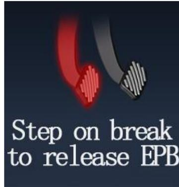
When the electronic handbrake is released without stepping on brake pedal, the indicator will prompt "Please step on brake pedal to release the electronic parking" for 5S, accompanied by a beep.
