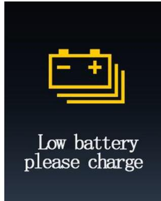
When SOC is less than 20%, the indicator lights up
