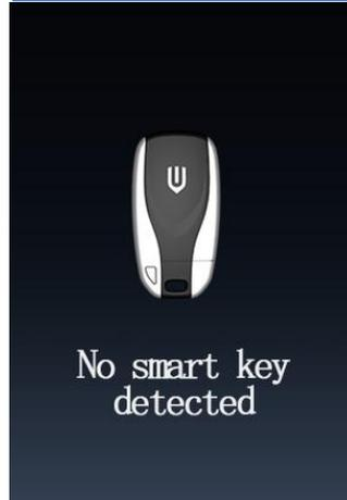
When smart key not detected, the meter will prompt "Smart key not detected" for 5s, accompanied by three beeps.
