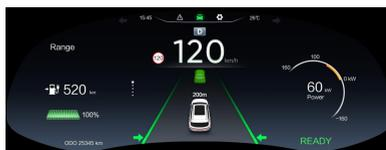
The Intelligent Cruise Assist function integrates adaptive cruise and lane centering functions, which can keep the vehicle in the middle of the lane and follow the preceding vehicle or drive at a constant speed when the vehicle is > 0km/h and the lane line is recognized.
