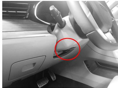
1. Push down the steering wheel adjustment handle;
