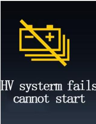
When the high voltage system is cut off and cannot be started, the indicator lights up
