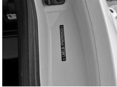
5. VIN code is located in the VIN slot on the left front side of the dashboard
