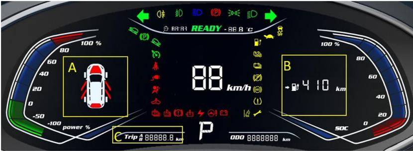
1. Press the "Instrument confirmation/return" button to switch related information display in area A (door opening prompt/tire pressure monitoring display area), area B (display area for average energy consumption, cruising range), and area C (subtotal mileage trip A, trip B). And when the subtotal mileage trip A or trip B in area C is selected, the subtotal mileage can be cleared by long pressing the "Instrument confirmation/return key".
