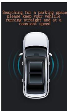
When the system finds the parking space, the interface will pop up "The parking space has been found, please stop" → "Please put P and leave the steering wheel with both hands" → "Please select the parking type and direction" interface, requiring the user to operate according to the system prompts.
