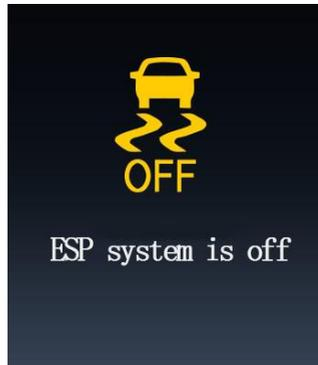
When the ESP function fails or the system is OFF, the indicator lights up the malfunction indicator
