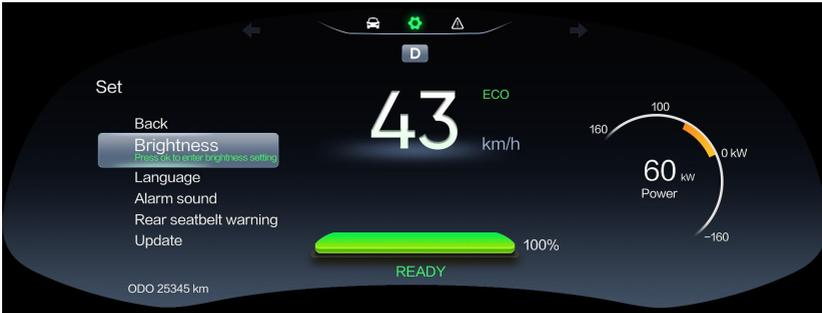
1. Press the "Instrument page up/page down" button to switch between "Settings", "Trip Computer" and "Fault Finding" menu items in the instrument menu selection area.
