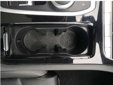
Pull the upper blade of the roller shutter backward to open the cup holder, and push the upper blade of the roller shutter forward until it is completely closed.
