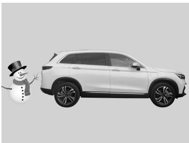
4. The radar probe may not be able to detect objects higher than the bumper.
