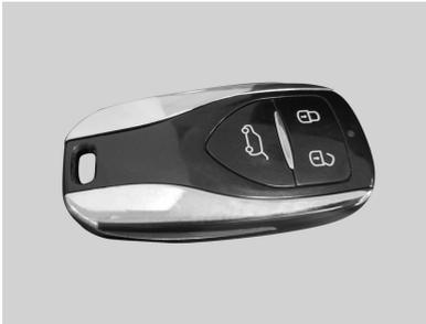
Carrying a remote control key, you can use the buttons on the remote control key to unlock/lock the door, open the tailgate, and find the vehicle.
