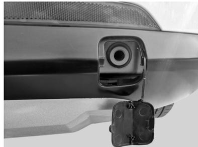
2. Install the tow hook into the tow hook hole in a clockwise direction, and then tighten it.
