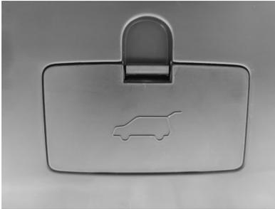
2. Tighten the tailgate emergency zipper, unlock and open the tailgate.
