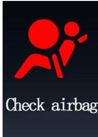
When the airbag function fails, the indicator lights up the airbag malfunction indicator
