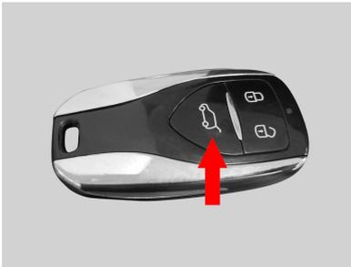
1. Long press the tailgate opening button on remote control key when vehicle power off;
