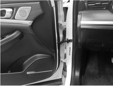
2. VIN code is located on the back side of the left front door panel
