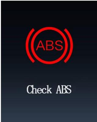
When the ABS anti-lock function is malfunctioning, the indicator lights up the malfunction indicator
