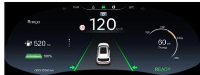
The lane keeping system is a system that assists in the correction of lightly deviated vehicles to ensure that the vehicle runs in the middle of the lane as much as possible, assists the driver to reduce traffic accidents due to lane departure, and improves driving safety.
