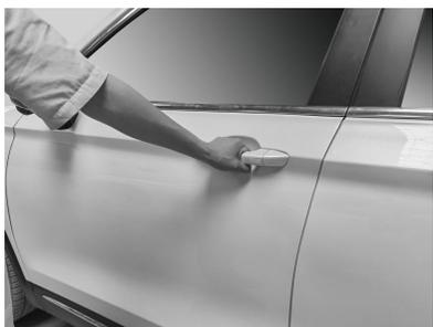
When the vehicle is powered off, bring the key to the front door within about 1 meter and hold the front door handle. After the sensor area inside the front door handle is effectively detected, the door is unlocked.
