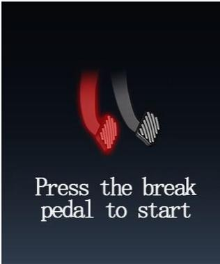
When the start button is pressed and the brake is not applied, the indicator prompts “Please depress the brake pedal to start” for 5s, accompanied by three beeps.
