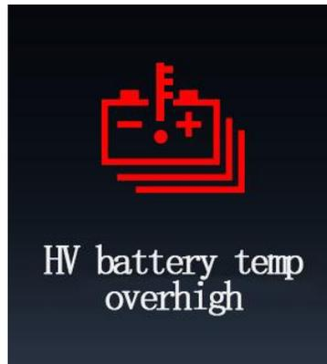
When the temperature of the power battery is too high and the power is reduced, the meter flashes red indicator
