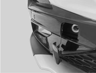
2. Install the tow hook into the tow hook hole in a clockwise direction, and then tighten it.
