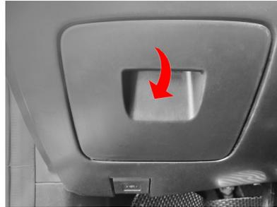
Pull the handle of the storage box backwards, and the storage box can be opened.
