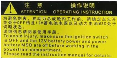
The warning label of the cooling fan is located on the inside front of the Front cabin
