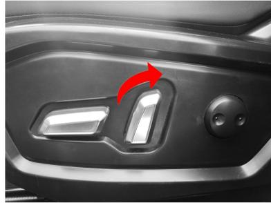
Adjust seat button2 in the direction shown in the figure to adjust the seat back angle.
