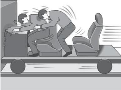
3 The person continues to move forward until blocked by an object. In actual vehicles, the object may be the windshield or dashboard or seat belt.
