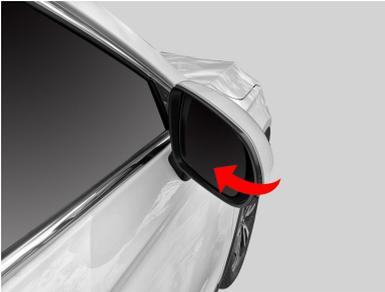
2. Operate the rearview mirror folding/unfolding button on the multimedia entertainment system (see the multimedia manual for details)
