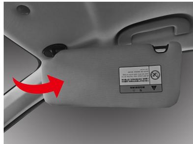
When closing the sun visor, you need to mount the sun visor to the fixed support and push it upward.
