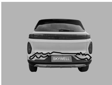
6. The radar probe is covered by dirt, snow or mud, etc., and may not be able to detect obstacles.
