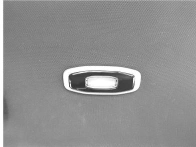
2. Open the door, the front and rear dome lights will automatically light up and go out after 1 minute, or the whole car will be powered off or locked, and the front and rear dome lights will go out immediately.
