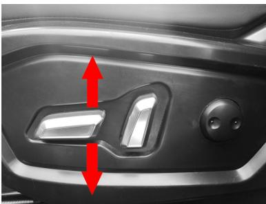
Adjust the rear part of the driver's seat button1 in the
