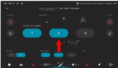
To operate the seat memory function, short press to call, long press to remember the current position.
