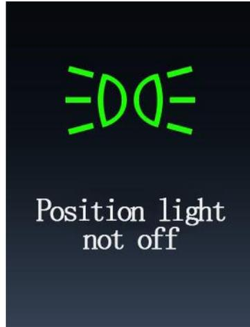
When the position light is not turned off, the meter will prompt "Position light is not turned off warning" for 10s, accompanied by an warning tone.
