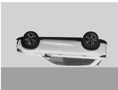
In the case of rollover, the side curtain may not be deployed.
