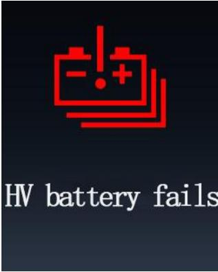
When the power battery malfunctions, the meter flashes (functionally limited)/steady light (emergency shutdown) red indicator
