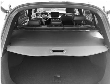
Pull out the cover curtain and clip both sides of the cover curtain into the fixing groove. When the cover curtain is not in use, just remove and retract it.
