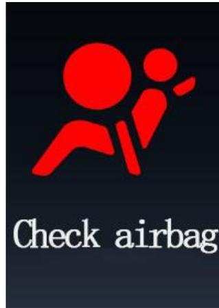
n KL15 ON state (ie D1 mode), when the airbag function fails, the indicator lights up the airbag malfunction indicator
