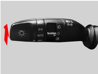
Move the light adjustment handle to the steering wheel and release, the high beam flashes once, and the high beam indicator on the instrument cluster assy flashes
