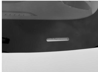
6. VIN code is located at the upper left end of the inner panel of the hood
