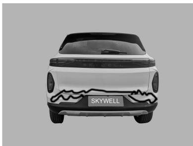
6. The radar probe is covered by dirt, snow or mud, etc., and may not be able to detect obstacles.
