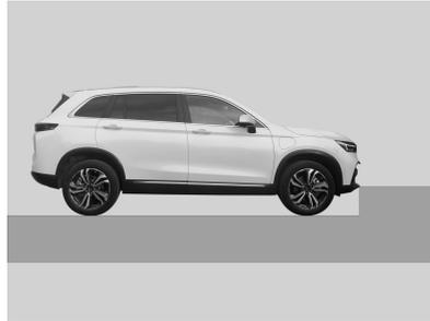
When the vehicle collides with low objects such as steps while driving, the airbag may not deploy. While the seat belt can protect your safety.
