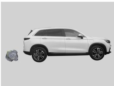
3. The radar probe cannot detect objects that easily absorb ultrasonic waves such as soft snow, cotton and sponges.
